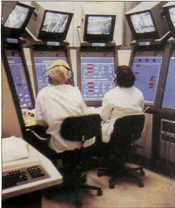
SIMULATING THE CONTROL SYSTEM BEFORE INSTALLATION LETS OPERATORS BECOME FAMILIAR WITH THE NEW ENVIRONMENT WHILE IT'S STILL RELATIVELY EASY TO MAKE CHANGES.
