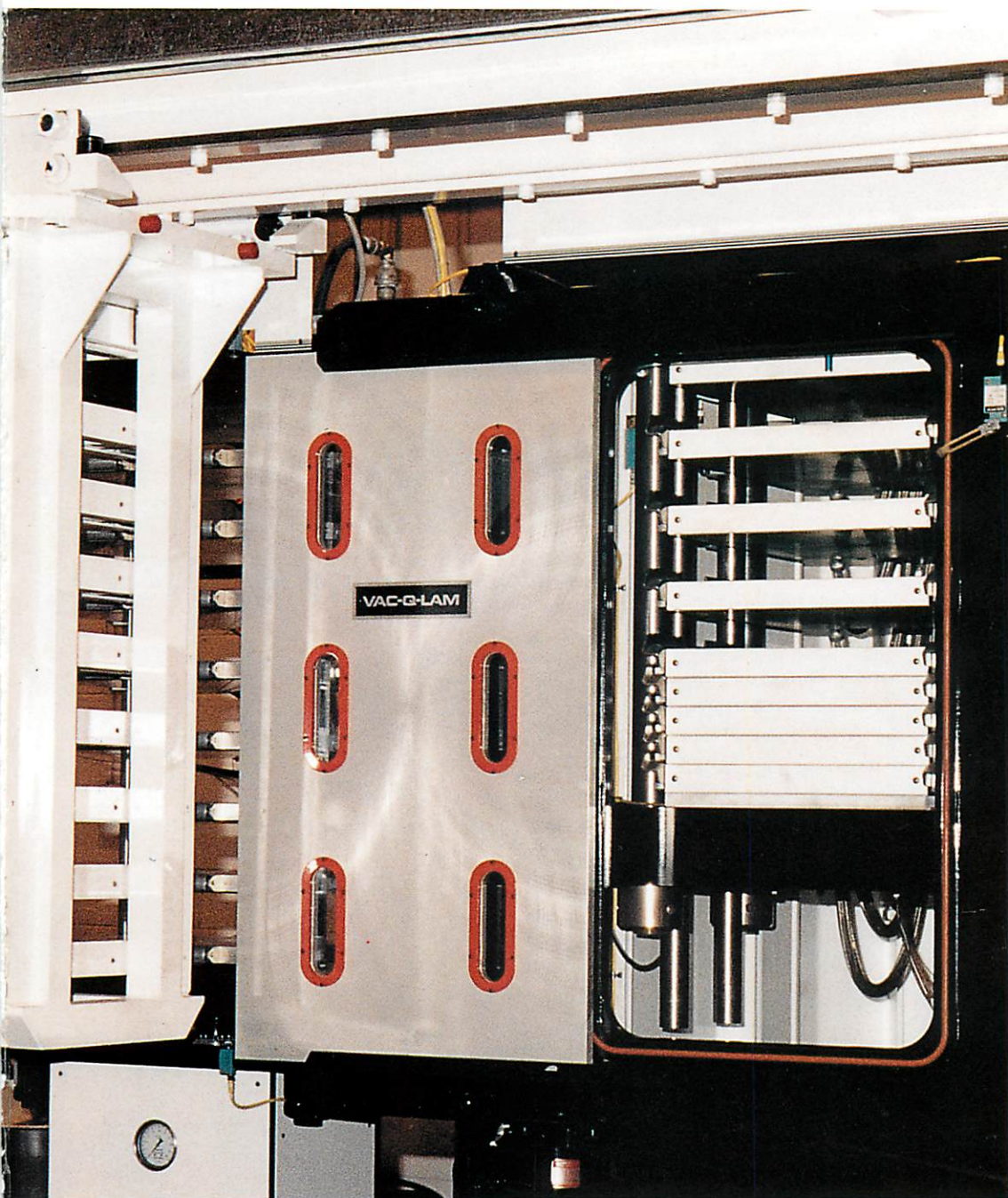
Smart Distributed System photoelectric sensors and limit switches were used on the equipment to determine if the doors to the presses were open or closed. Proximity sensors were used to detect the presence or absence of parts in the mold.
