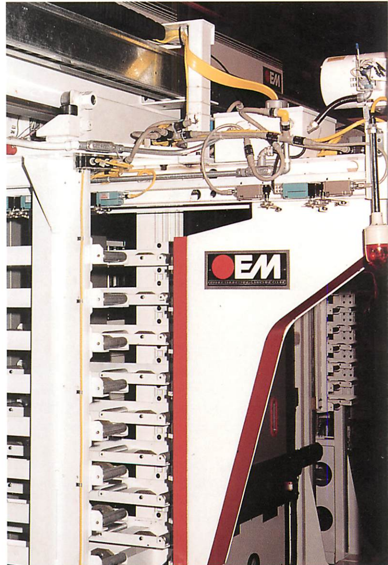
The equipment used in the installation was fully automatic, including the gantry system which loads and unloads the presses.
